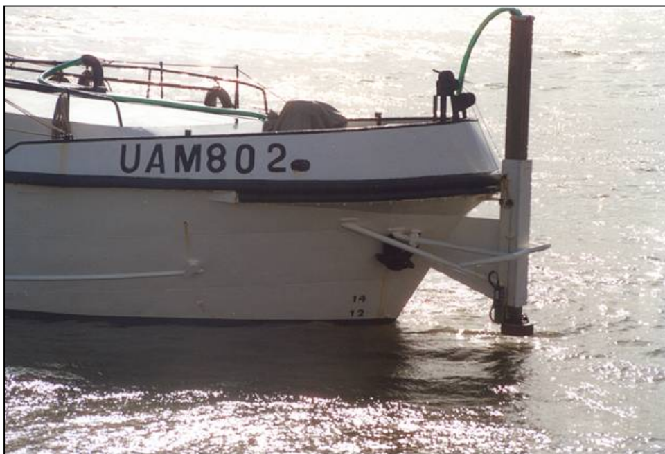
Fig. 3.19 "Transducer installation over the bow"
